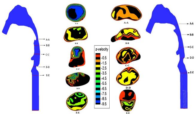
Fig. 1 Flow visualization in upper airway of OSA patient pre-surgery (left) and post-surgery (right).
