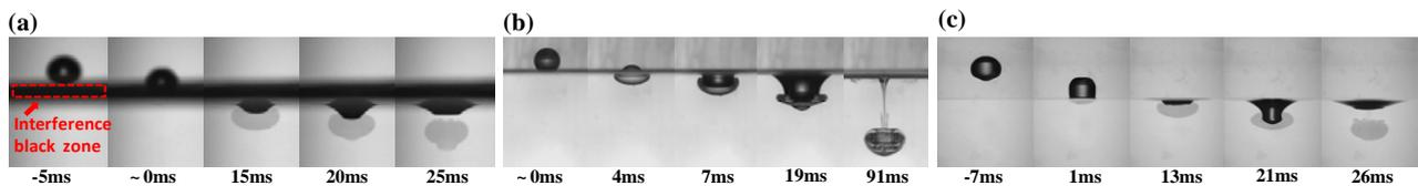
Fig. 1 The development of vortex ring by (a) water drop (drop diameter  $D=5.52\text{mm}$ , impact height  $H=24\text{mm}$ ) and (b) 60% glycerol mixture ( $D = 3.69\text{mm}$ ,  $H = 24\text{mm}$ ) impacting onto water target liquid, (c) water drop (drop diameter  $D=5.52\text{mm}$ , impact height  $H=22\text{mm}$ ) with special control of meniscus interface.
