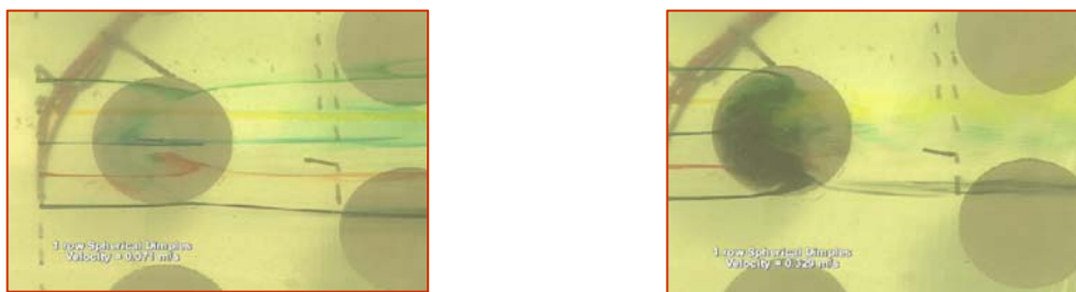
Fig. 1 Flow visualization for the one-row of spherical dimples. a: water speed is 0.071 m/c, b: water speed is 0.33 m/c (here the second row is «closed» by means of plastic material).
