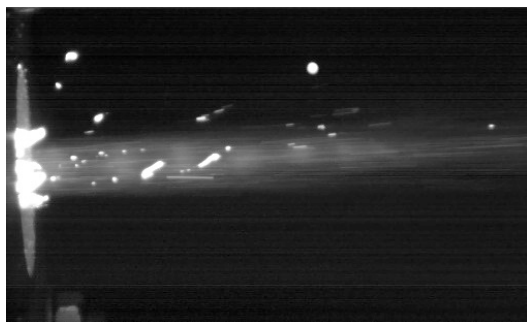
Fig. 1. Flow visualization of spraying process in supersonic plasma jet.
