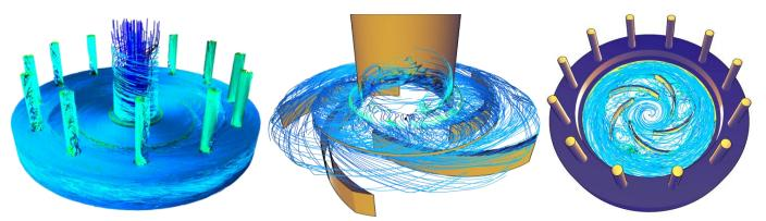
**Figure 4**: Path line visualization of particle trajectories for all 80 time steps. Color encodes the magnitude of the particle movement in z direction, while cyan indicates particles moving upwards, and dark blue particles moving downwards.
