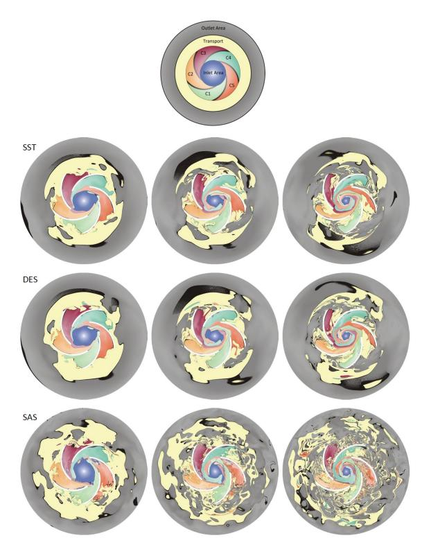
**Figure 7:** Using advection of a given input texture clearly shows the resulting transport into the channels after 20, 50, and 80 time steps. Using forward advection the visualization efficiently encodes which areas end up in a specific channel after the advection time.
