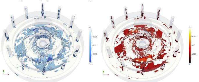
**Figure 2**: The image shows the  $\lambda_2$  (left) and Q criterion as 3D iso-surfaces for the SAS model. The resulting structures are delicate and complex due to the high degree of turbulence in the velocity field. Further, they only describe one single time step ( $t_0 = 0$ ), while a structural overview requires the consideration all time steps.
