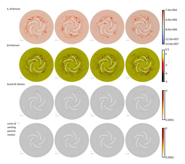
**Figure 3:** Comparative overview of different vortex criteria for the SAS Model (time steps 0, 25, 50 und 80).  $\lambda_2$  vortices are defined as dark red iso-levels, Q as dark yellow regions. The last two criteria define binary maps, where dark spots mark potential vortex core line positions.
