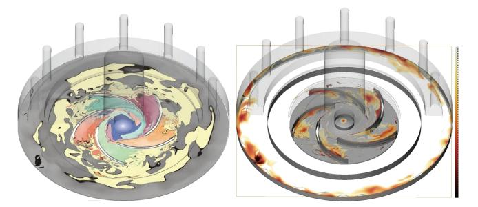
**Figure 9:** Both image illustrate two global measures in the geometric context of the pump. The left image illustrates the advected channels of the SAS model until time step 50. On the right side stagnating flow areas are emphasized, which effectively communicates blocked channels.
