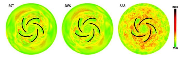
**Figure 5:** Comparative visualization of the FTLE field for all three simulation models with tau=80. Locally high FTLE values denote large particle separation, while low values indicate trajectories staying close over the considered time interval, which emphasizes potential backflow areas.
