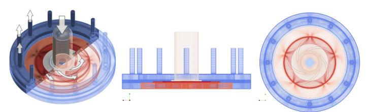
Figure 1: The left image shows the functional parts of the pump together with principle flow directions. The remaining images show side and top view with outlet and impeller sections of the transport area.
