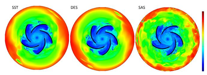
**Figure 6:** Comparative visualization of the accumulated velocity field for all three simulation models with tau=80. Locally low values denote regions of stagnating flow and lower particle velocities. This becomes especially apparent in the center of blocked channels.
