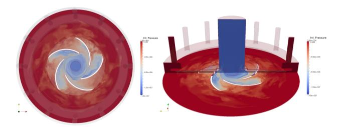
**Figure 8:** Integrated pressure for the SAS model over the complete temporal domain. Locally minimal regions (blue) indicate areas of recirculation and stagnating flow.
