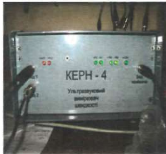
Fig. 2 The window illustration of data treatment of elastic waves velocities measuring by the echo-impulse method on frequency f_{||} \approx 1,11 MGz, f_{\perp} \approx 0,43 MGz and appearance of computer device KERN-4
