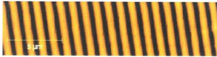
Fig. 8. AFM image of recorded holographic grating
