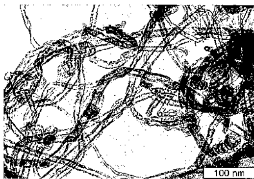
Fig. 4. Carbon nanotubes obtained at the A. V. Luikov Heat and Mass Transfer Institute
